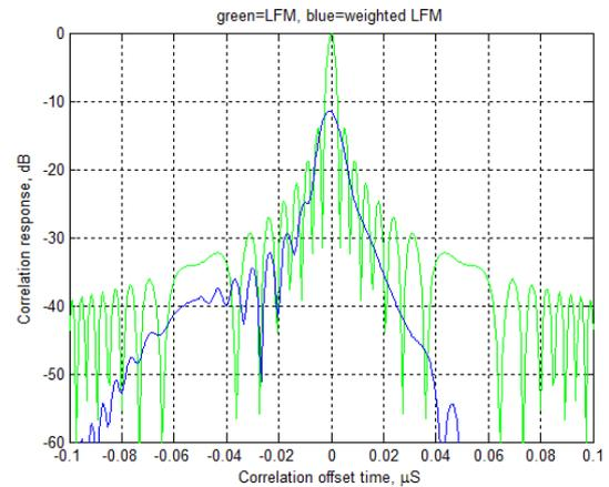
Figure 2: Cross correlation profile showing effect of 50% trailing-edge eclipsing for a Linear FM chirp with a Hamming window function.
