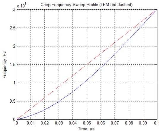
Figure 4: Optimised Non-Linear FM frequency sweep profile. Sweep profile optimised for eclipsing of leading left-side section only. Red dashed line shows reference LFM sweep.
