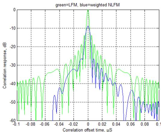
Figure 7: Cross correlation profile showing effect of 50% eclipsing for an optimised Non-Linear FM chirp with a window function optimised to tolerate eclipsing of one edge only.
