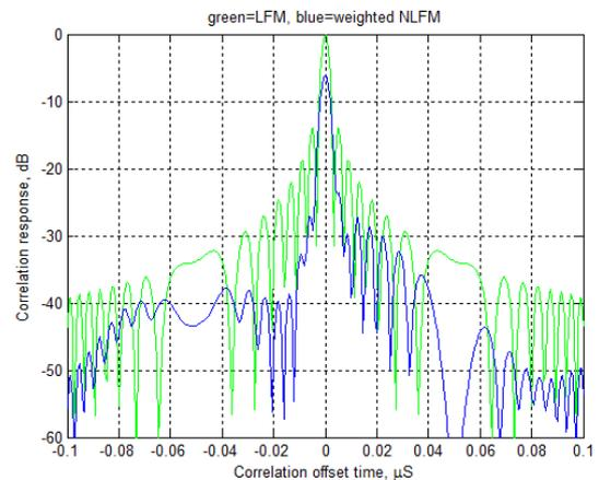
Figure 6: Cross correlation profile showing effect of no eclipsing for an optimised Non-Linear FM chirp with a window function optimised to tolerate eclipsing of one edge only.
