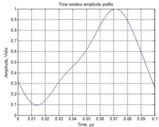
Figure 5: Optimised window function profile. Window function is optimised in conjunction with the non-linear frequency sweep to tolerate eclipsing of left edge only.
