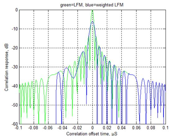
Figure 1: Cross correlation profile showing effect of 50% leading-edge eclipsing for a Linear FM chirp with a rectangular window function. Green line shows reference un-eclipsed LFM with rectangular window.
